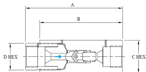
BuTech ball check valves prevent reverse flow where leak-tight shutoff is not necessary. The valves are made from 15-5PH stainless steel with 17-4PH poppets for long life and 303 series stainless spring.
